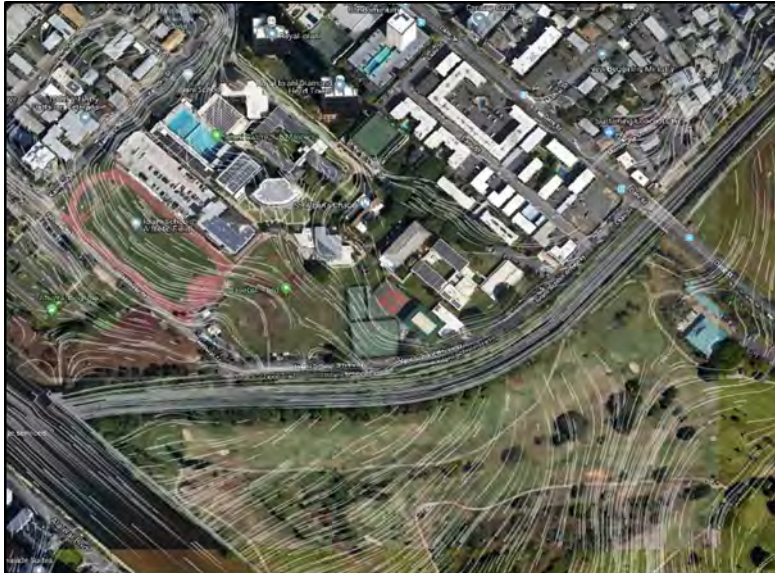
Figure 32: Storm water flow direction and velocity Without Project (1% AEP) at confluence of M-P and Ala Wai canal
