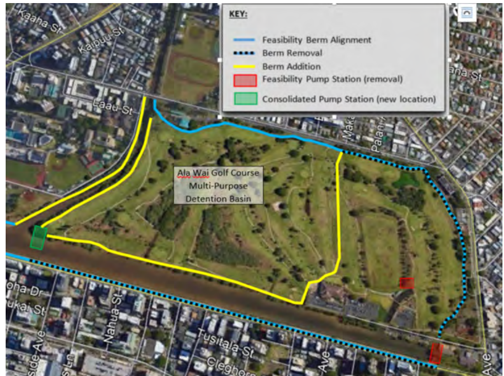
Figure 28: Flood barrier system alignment and modifications at the Ala Wai Golf Course
