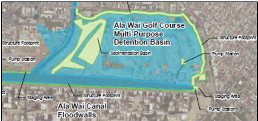
Figure 27: Golf course detention basin berm alignment on north and east sides as designed during Feasibility
