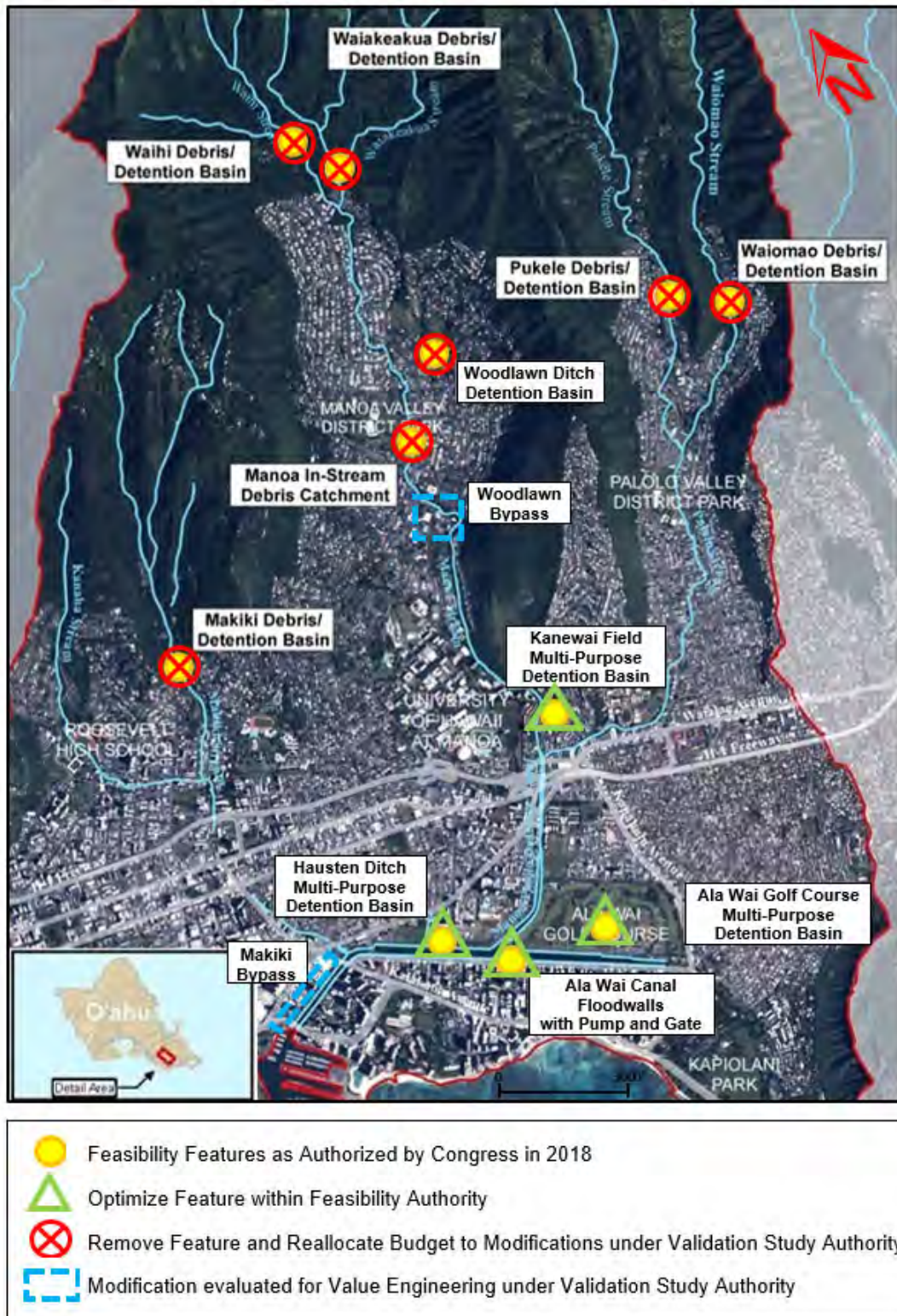
Figure 36: Recommended modifications to the authorized FFEIS Project as detailed in this Engineering Documentation Report
