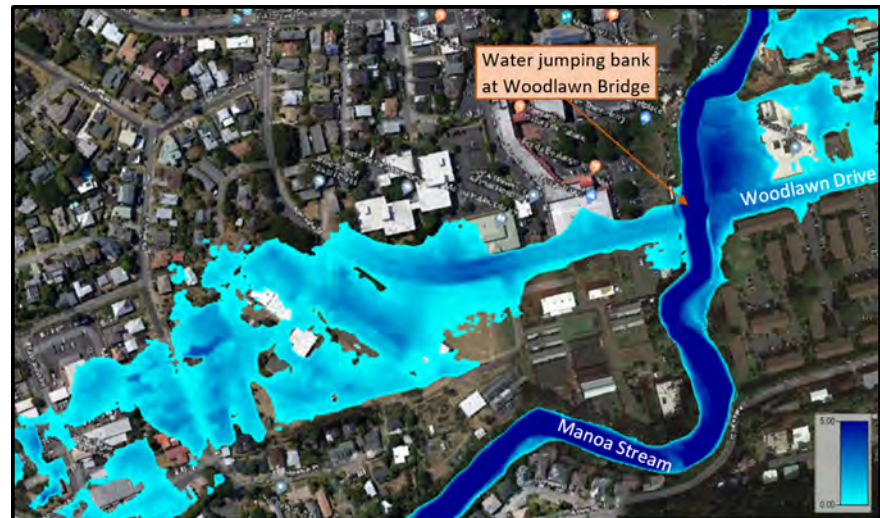
Figure 17: HEC-RAS 1D/2D modeling results with Waihi and Waiakeakua optimized illustrates water still jumps bank at Woodlawn Bridge, 1% AEP.
